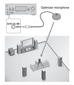
Connect the supplied optimizer microphone to the AUTO CAL MIC jack on the front panel.
